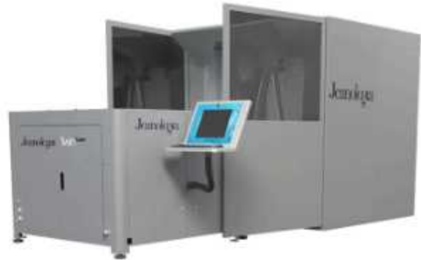
Figure 6: Laser-based machine for denim textile (5)
