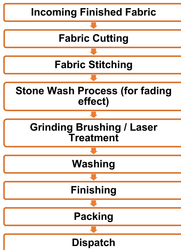
Fig. 3.1: Process flow for denim fabric/garment processing
