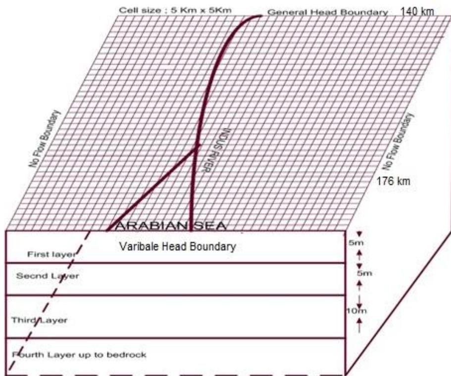
**Fig. 3.42: Surface-cum groundwater interaction model**
