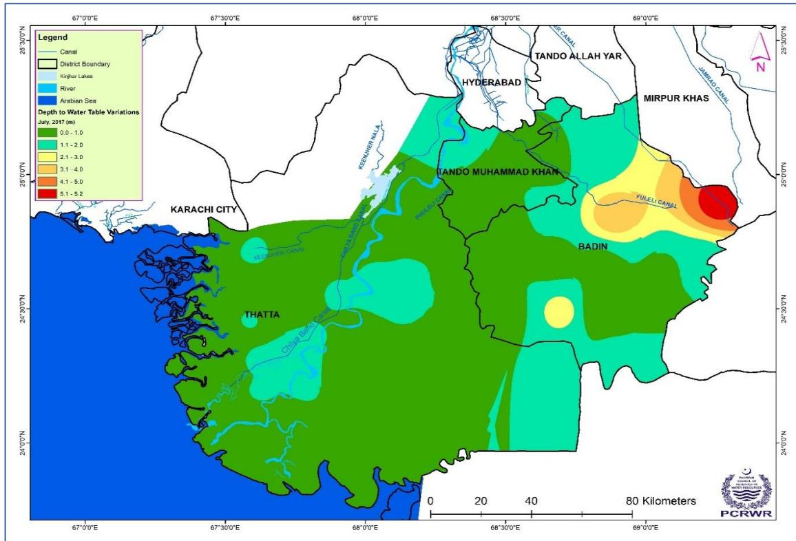
**Fig. 3.3: Depth to water table during July-August 2017 in the Indus delta**
