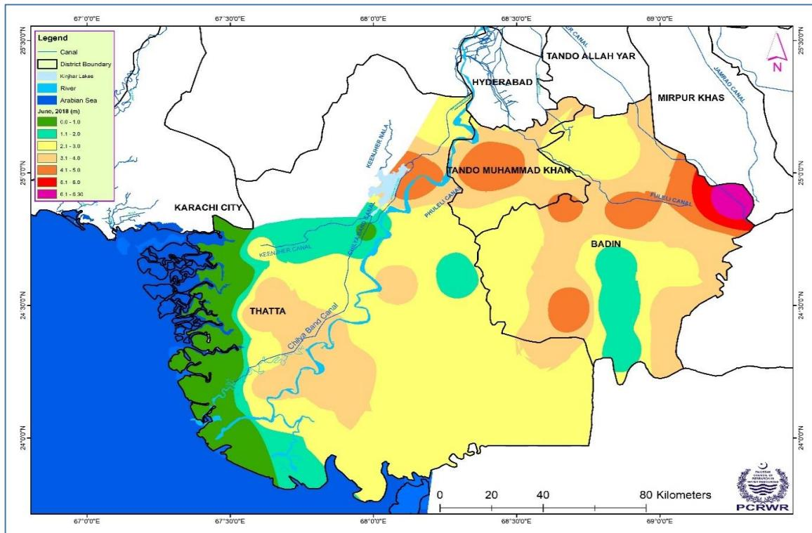
**Fig. 3.4: Depth to water table during June 2018 in the Indus delta**
