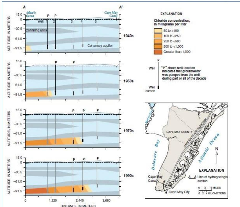
**Fig. 3.20: Hydrogeologic sections showing lateral concentration of saltwater (chloride) and contamination of supply wells in the Cape May City (New Jersey) well field , Coastal region, North America from 1940 to 1990 (Source: Barlow and Reichard, 2010)**
