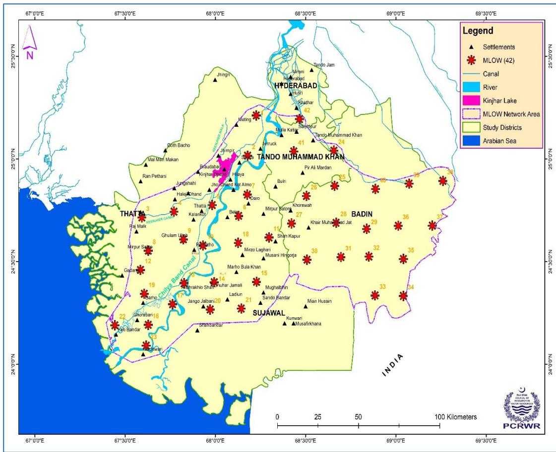
**Fig. 2.2: Piezometric network developed under study for groundwater quality and levels**
