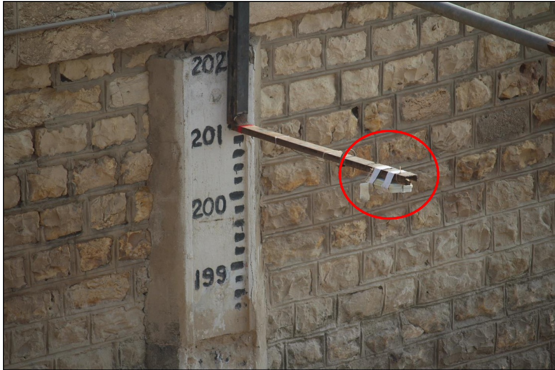
Fig. 2.7: Real-time water level sensor
