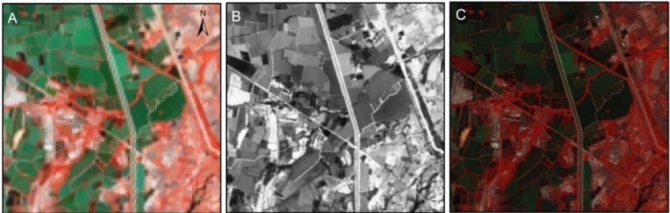
**Fig. 6** Visual comparison of spatial resolution using **a** Landsat color composite image of 30 m, **b** panchromatic band of OLI sensor of 15 m and **c** RapidEye color image of 5 m
