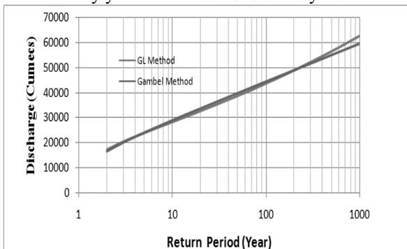
Fig-7: Computed Return Period (in years) at Guddu Barrage by both Generalised Logistic (GL) and Gambel Methods.
