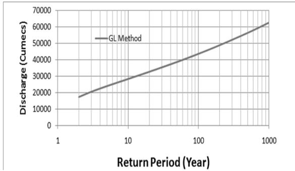
Fig-6: Return Period (in years) at Guddu Barrage computed by Generalised Logistic (GL) method.
