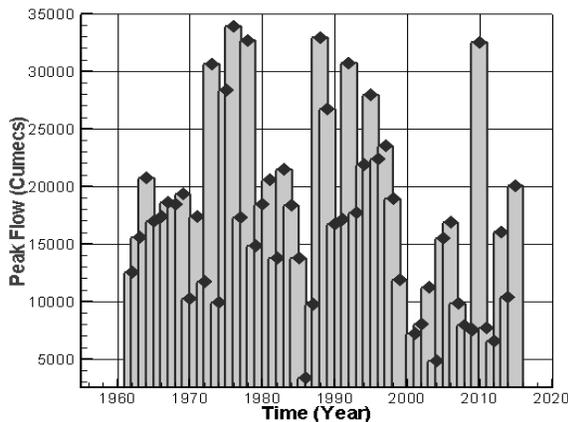
Fig-2: Flood Peaks Flow at Guddu barrage.
