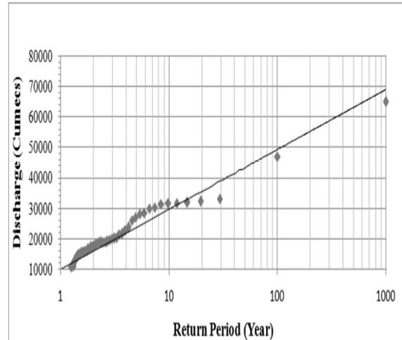
Fig-8: Return Period (in years) at Sukkur Barrage computed by California method.
