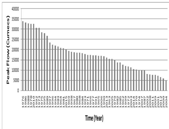
Fig-3:Peak Flows from (Supper to Normal Floods) at Guddu barrage.
