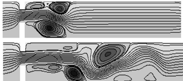
Fig.3: Streamline pattern, at Re=10, for non-dimensional time units  $t=100$  and  $300$ .
