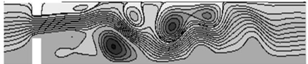
Fig.4: Streamline pattern, at Re=15, for non-dimensional time unit  $300$ .
