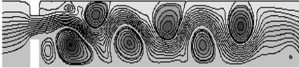
**Fig.6: Streamline pattern, at  $Re=50$ , for non-dimensional time unit 300.**
