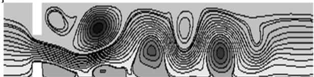
Fig.5: Streamline pattern, at Re=25, for non-dimensional time unit  $300$ .
